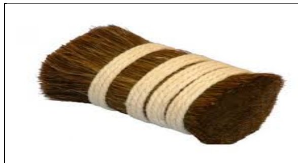
Figure 4.1 Horsehair used in concrete
