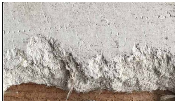
Figure 4.2 Asbestos used in ancient concrete
